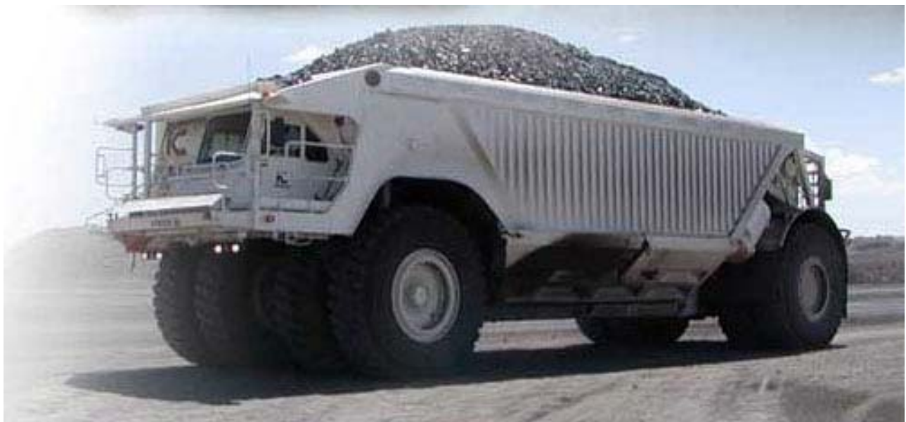
Figure: A bottom dump coal hauler manufactured by Kress.
